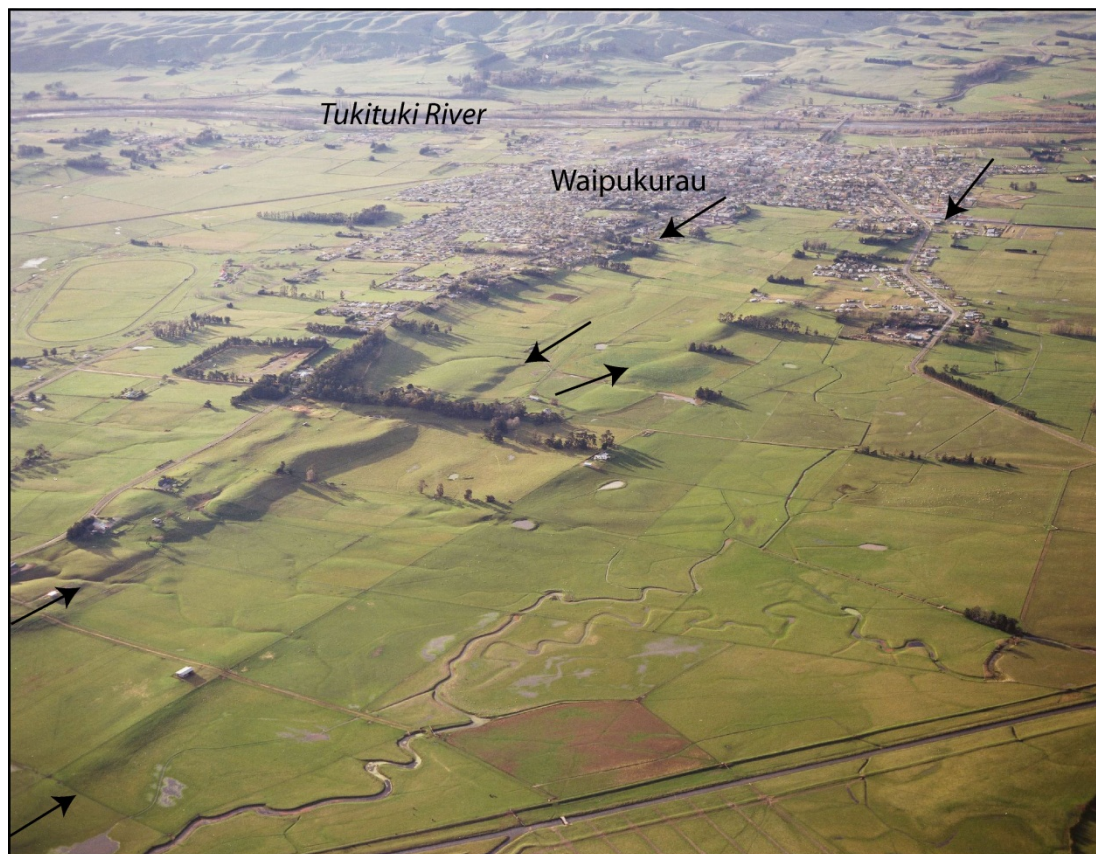
Figure 3.7 Oblique aerial photograph of the Waipukurau Fault Zone, south of, and including Waipukurau township, and toward the Tukituki River. The fault zone comprises a series of parallel and stepping anticlinal ridges (scarps) formed on the upthrown side of reverse faults (Photo: Lloyd Homer, GNS Science).
