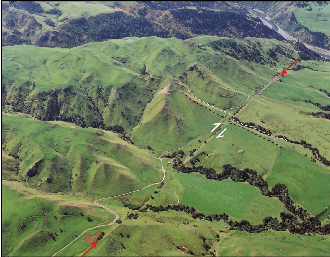
Figure 3.2 View to the north along the Mohaka Fault, just to the south of the Ngaruroro River (pictured) near Kereru. The active trace of the fault is marked by red arrows, and the sense of movement across the fault is highlighted by white arrows. A pair of offset features (a stream and adjacent ridgeline) are highlighted (dashed lines) to illustrate the right-lateral movement across the fault.
