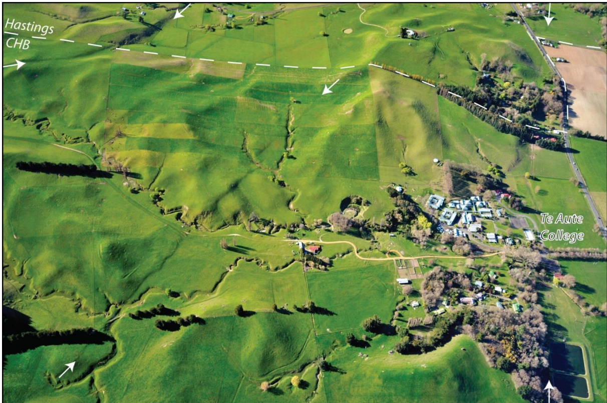
Figure 4.6 Geomorphic expression of the Poukawa Fault Zone at the southern edge of Hastings District, in the vicinity of Te Aute College. Three parallel zones of active reverse faulting are indicated by white arrows. State Highway 2 is at right (Photograph: D. Townsend, GNS Science).
