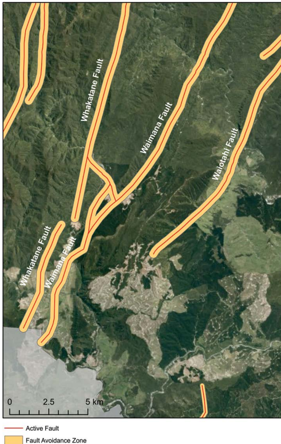
Figure 3.1 Detail of the Whakatane Fault and Waimana Fault in the southern part of the Wairoa District. Revised line work in this report and Fault avoidance Zones
