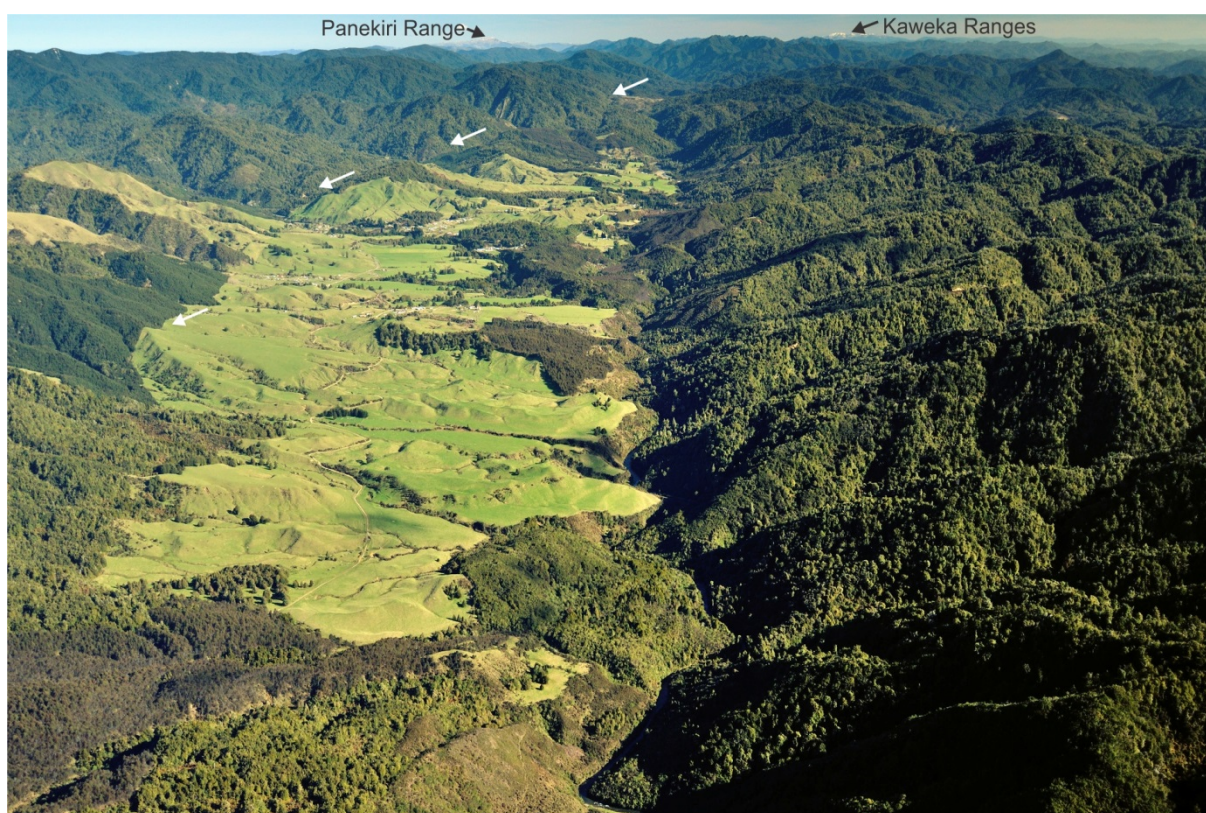
Figure 2.4 Oblique aerial photograph of the Whakatane Fault (white arrows point to fault trace) running through the Ruatahuna basin. The photo perspective is looking southward toward the Wairoa District. Photo credit: Dougal Townsend, GNS Science.
